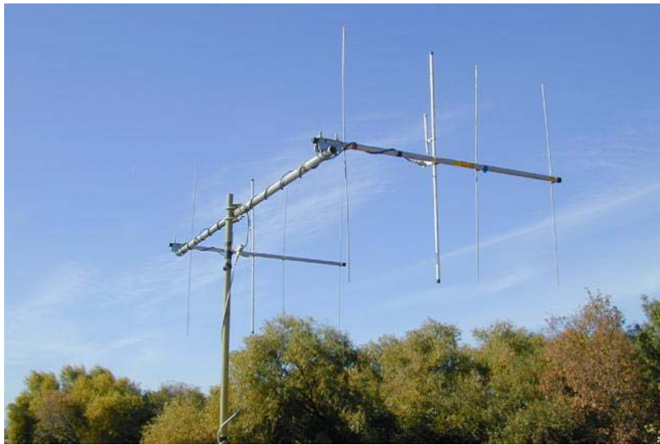
Figure 11. Five-element precision direction finding arrays (Model RA-NS, Telonics). ESRP photo.
