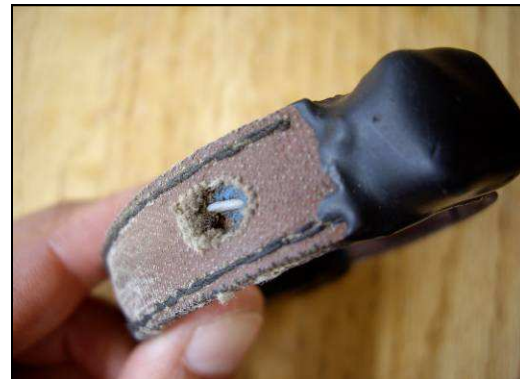
Unit 2441.3809 – Antenna broken at collar.
