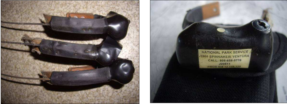
Figure 5. Typical wear observed on proximity logger units deployed on San Miguel island foxes in 2009-2010.
