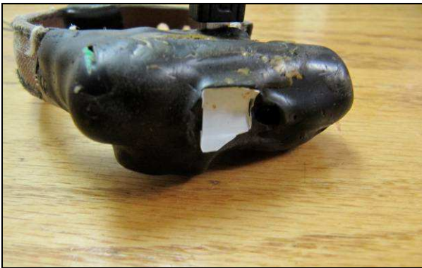
Unit 2451.3109 – Broken housing.
