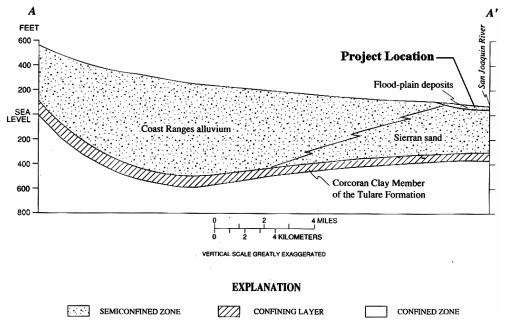
Figure 13. Generalized hydrogeologic cross section in the Land Retirement Demonstration Project vicinity. (Modified from Belitz and Heimes, 1990).
