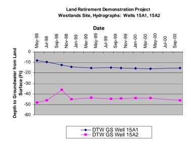
Figure 17. Hydrographs for monitor wells 15A1 and 15A2 showing typical vertical hydraulic gradients measured at the site. DTW GS = Depth to Water from Ground Surface.
