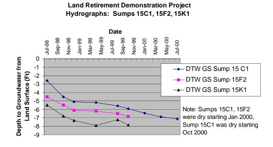
Figure 19. Hydrographs for three agricultural drain sumps at the Westlands Site showing a declining shallow groundwater trend. DTWGS = depth to water from ground surface.
