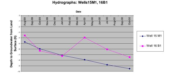
Figure 21. Hydrograph for monitor wells 15M1 and 16B1 at the Westlands Site showing and overall declining shallow groundwater trend.
