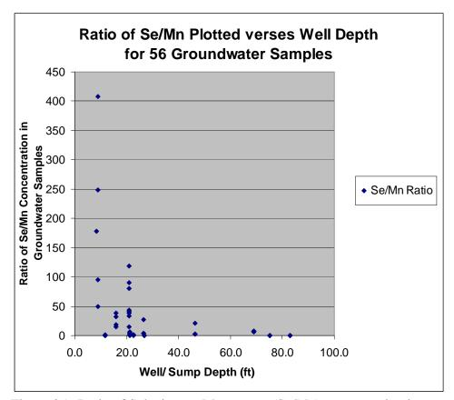
Figure 25. Ratio of Selenium to Manganese (Se/Mn) concentration in groundwater samples plotted verses well depth. The Se/Mn ratio shows a decreasing trend with depth indicating oxidizing geochemical conditions in the shallow wells and reducing conditions in the deep wells.
