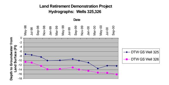
Figure 20. Hydrograph for monitor wells 325 and 326 at the Westlands Site showing typical vertical hydraulic gradient and the declining shallow groundwater trend observed.
