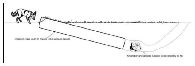
Figure 17. Alternative den design using a single length of irrigation pipe.
