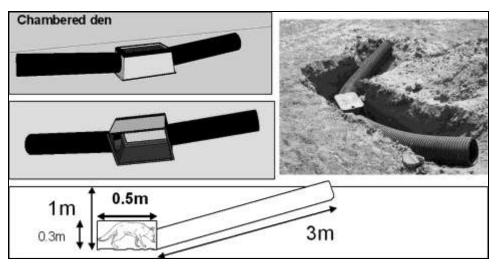
Figure 2. Schematic and field example of subterranean chambered den for kit foxes.
