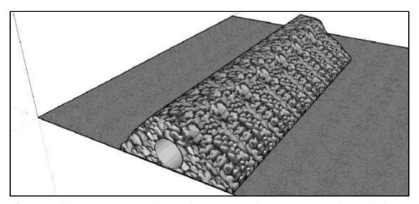
Figure 19. Heavy substrate such as rocks can be used to cover escape dens and thus prevent livestock from exposing the structure to the elements.
